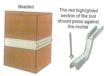
Assuming that the piers are stable enough to repair in place, the method would be to rake or cut out mismatched mortar and any unstable stone or mortar, to replace river cobble in-kind, and to re-mortar with a mortar mixed matching the extant original areas in color, grain, and beaded tooling.
